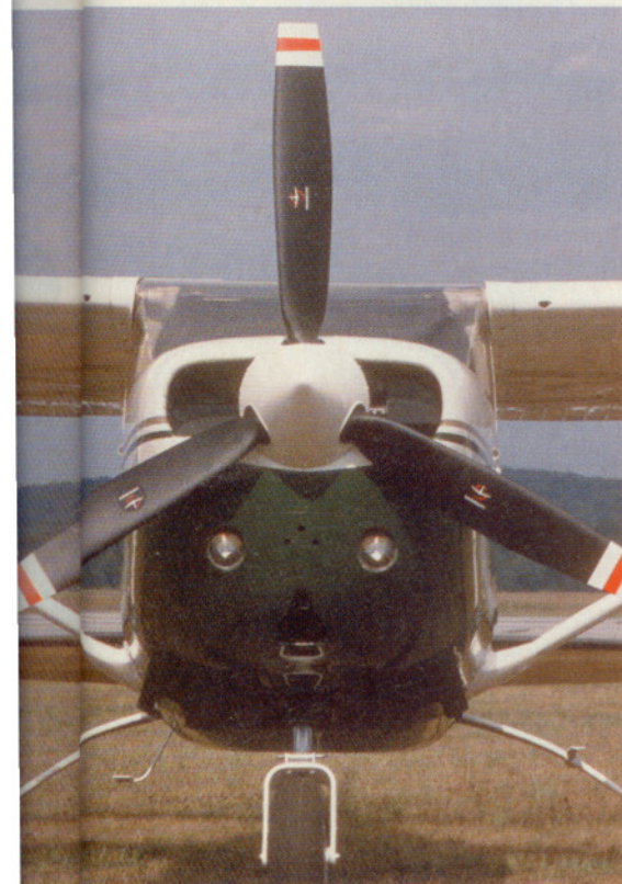
The original Continental IO-520 has been supplanted by a new Platinum-series IO-550 with more power and a longer warranty.
